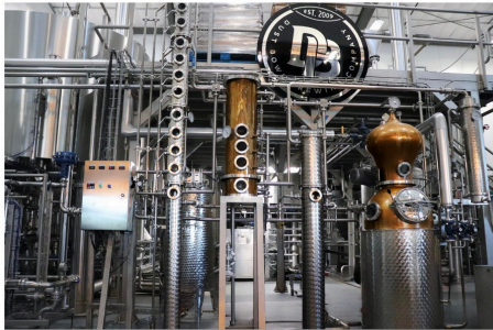
Described as a boutique operation, Dust Bowl Distillery features a 140-liter CARL still enhanced by the addition of a vodka column and gin basket from Minnetonka Brewing Equipment, allowing for a broad range of spirits to be produced. It is visible to guests through the taproom's bar windows (Photo contributed).
